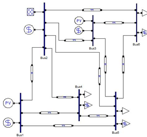
**Figure 4: Six Bus Test System**
