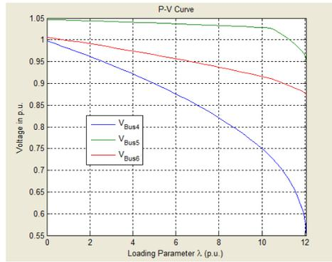
Figure 10: PV Curve (bus5)
