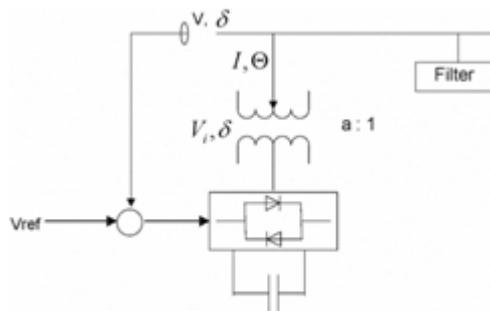
**Figure 3: Basic Structure of STATCOM**
